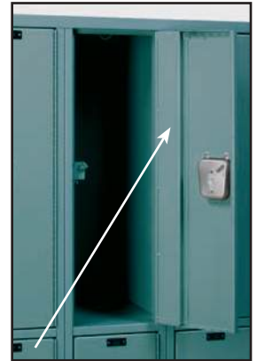
Hallowell HSPS-05 lockers include a 3" wide 18 gauge full height door stiffener spot welded to the inner door face and MIG welded to the hinge side as well as to the top and bottom door flanges providing a rigid torque-free door. A 1-1/2" wide stiffener will be furnished for 9" wide HSPS-05 doors.
